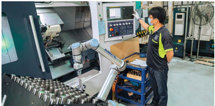
A UR10e cobot is deployed for loading parts into, and unloading parts from, the CNC machine.
