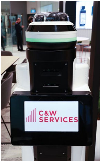
A security robot, equipped with AI vision analytics that supports security and facility inspection, was used to enforce Safe Management Measures during the COVID-19 pandemic.
