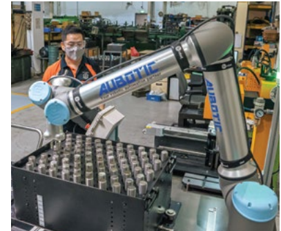
A UR10e cobot engraving part numbers and information on steel bolts.
